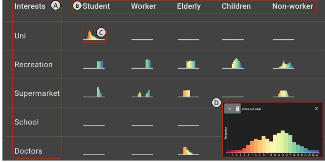
Fig. 3: The Scenario Editor to modify the mobility profiles of different demographic groups (B). For each demographic, different categories of interest (A, i.e., one or more different POI types) are modeled with a probability of visit (C) for a particular time of day within a prototypical week. The inset (D) shows a more detailed example.
