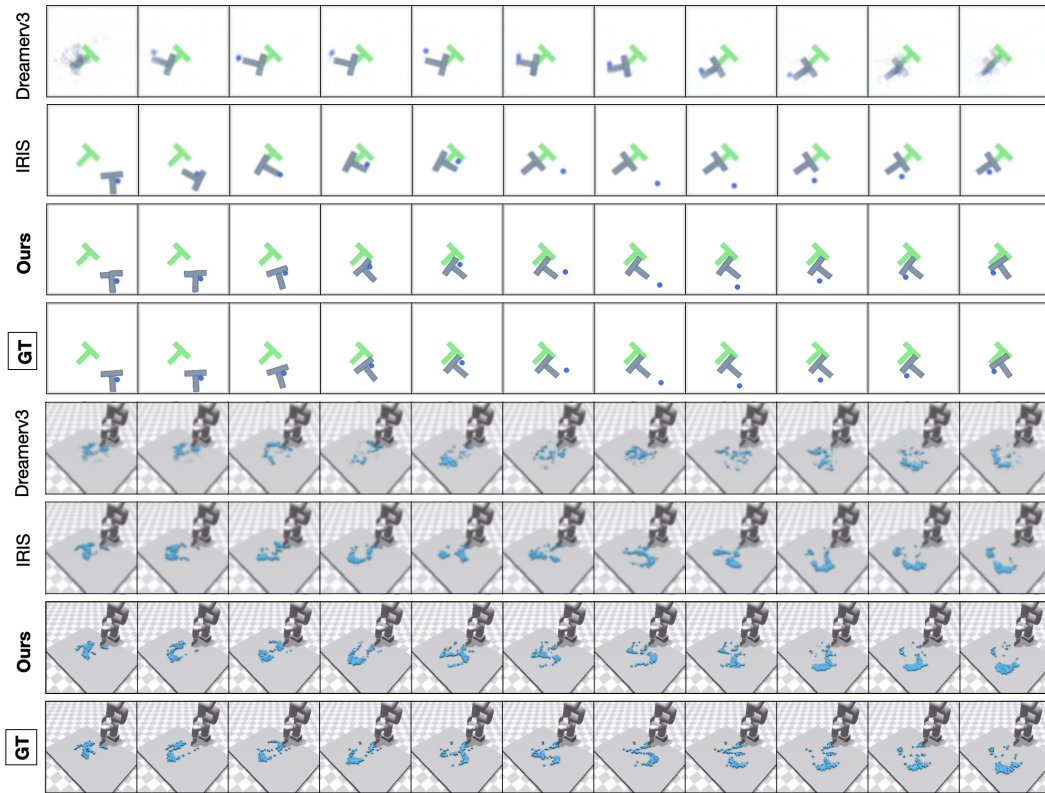
Figure 4: Openloop rollout of world models trained with various pre-trained encoders on Push-T and Granular environment. For each trajectory, the model is given the first frame as well as sequence of actions. The world models performs openloop rollout with these actions, and the images are reconstructed by a pre-trained decoder. For each environment, the bottom row denotes the ground truth. DINO-WM (Ours) rollouts are bolded and are visually indistinguishable from the ground truth observations.
